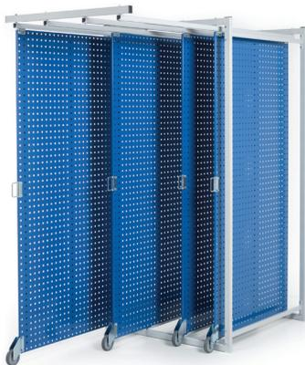
The TKT tool storage system requires only 21.5 ft<sup>2</sup> of floor space and provides 172 ft<sup>2</sup> of storage space. There is no need to attach it to the floor, as it stands firmly on its own. There is a castor on the lower edge of the panels which makes them easy to move.
